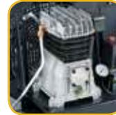
Lubricated 2 HP pump with cylinders in cast iron.
