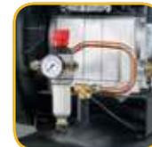
Pressure regulator with dual compressed air output.
